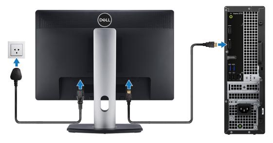
() **NOTE:** The location to connect the display cable can vary if your computer has a discrete graphics card installed. For optimal graphics performance, ensure to connect the display cable to the graphics card if there is one installed.
